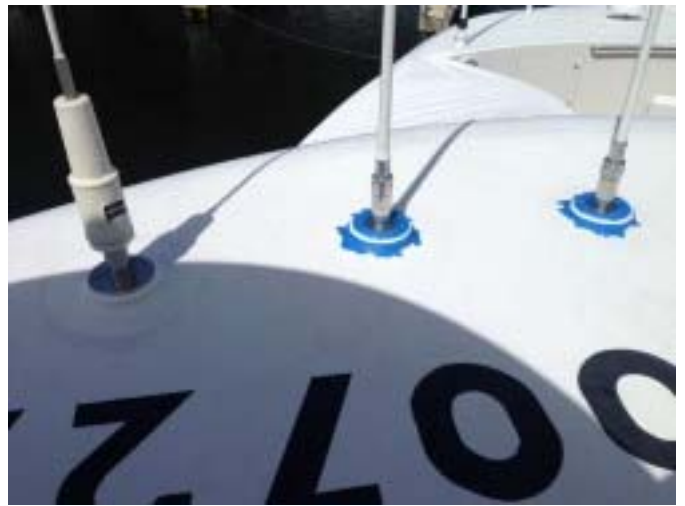
New Antenna Mounts
