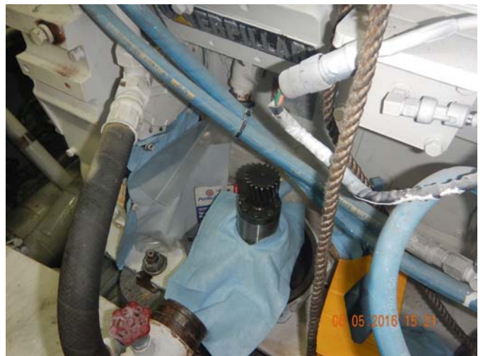
Main Engine Water Pump Change
