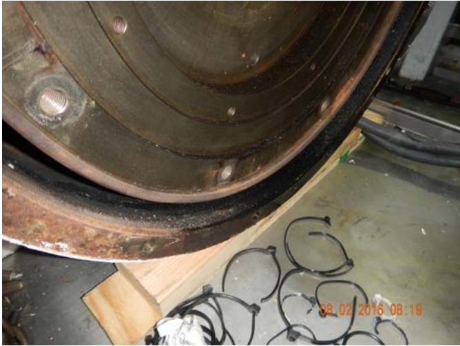
Main Oil Seal Leak on # 3 Generator
