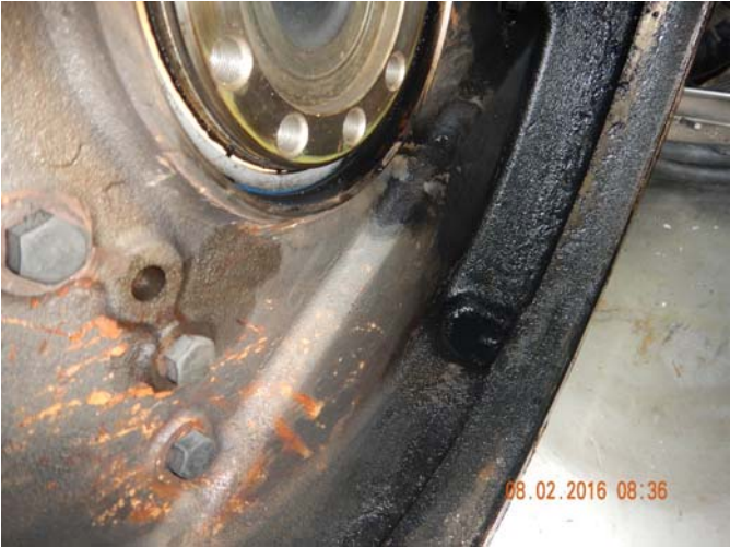
Main Oil Seal Leak on # 3 Generator
