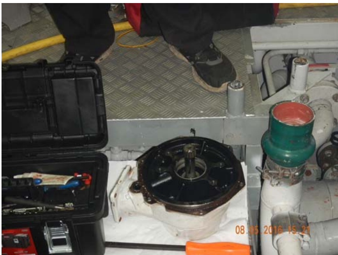
Main Engine Water Pump Change
